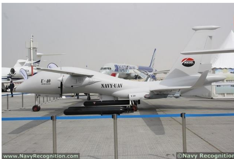
Figur 18: Navy ASW-UAV : Under Dubai Air Show i 2013 ble det vist frem en prototyp for en mulig MALE (Medium Altitude Long Endurance) ASW-UAV (kilde: www.navyrecognition.com ).
