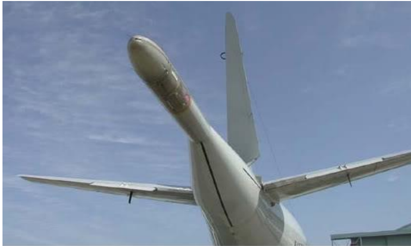
Figur 4: MAD-sensoren på et P3 Orion (kilde: http://harp gamer.com/harpforum/index.php?/topic/3527-tactics-101-anti-submarine-warfare-asw-part-2/ )
